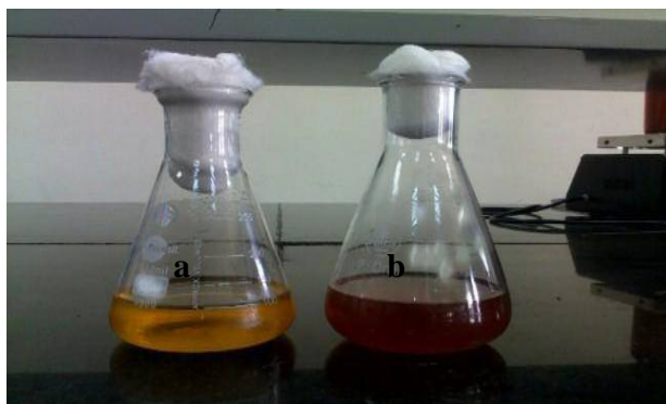
Figure 1: Flasks containing the Psidium guajava leaves extract before (a) and after (b) incubation in an aqueous solution of AgNO 3 solution.
